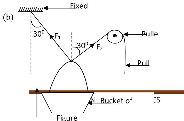
Figure 3 shows a bucket of sand which is pulled upward at a building site at the instant shown, the forces  $F_1$  and  $F_2$  have equal magnitudes of 600 N and the bucket is moving with an acceleration of  $2 \text{ ms}^{-2}$ . Determine the mass of the bucket and its content.
