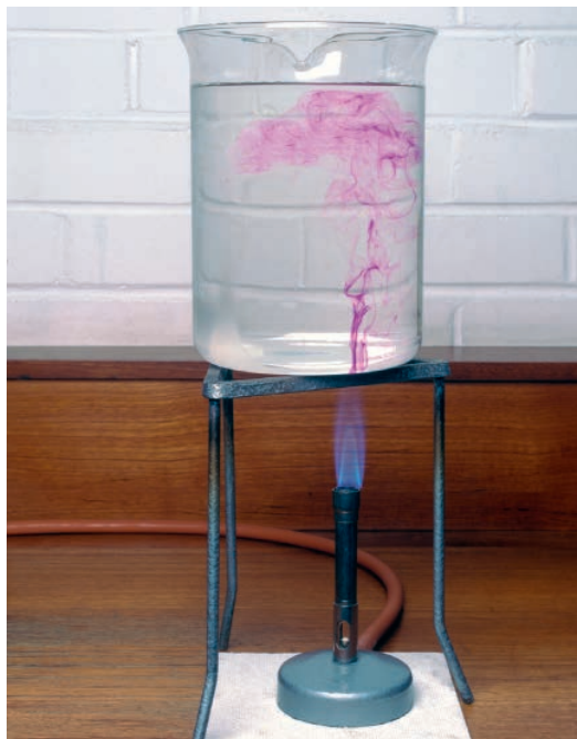
▲ Figure 2.3.4a Convection currents shown by potassium permanganate in water.
