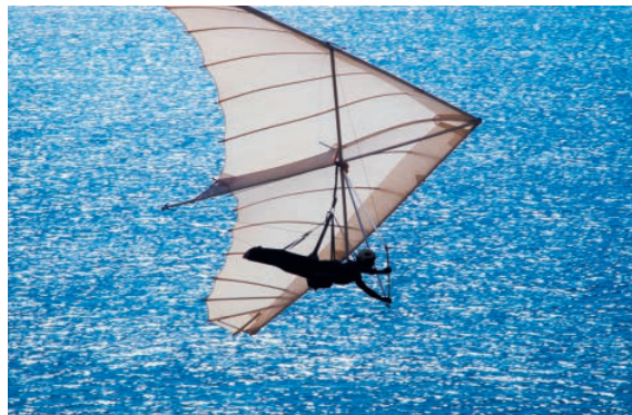
▲ Figure 2.3.7 Once airborne, a hang-glider pilot can stay aloft for several hours by flying from one thermal to another.
