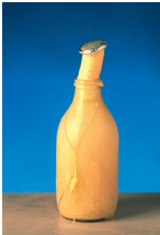
▲ Figure 2.2.7 Result of the expansion of water on freezing
