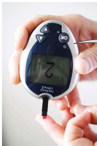
Figure 14.13 Biosensor for blood glucose testing
