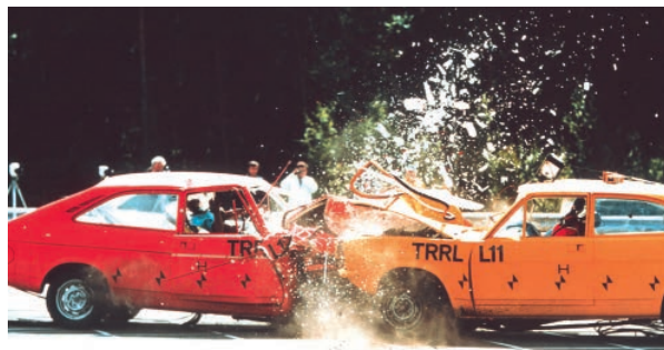
▲ Figure 1.7.11 Cars in an impact test showing the collapse of the front crumple zone
