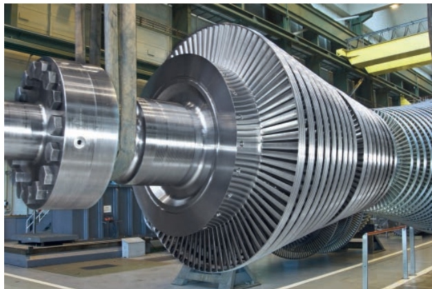
▲ Figure 1.7.19 The rotor of a steam turbine
