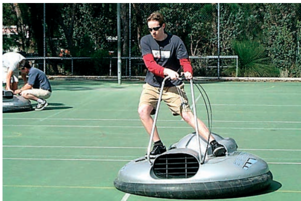
▲ Figure 1.5.8 Friction is much reduced for a hover scooter.
