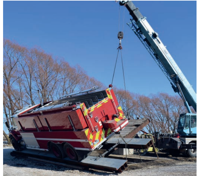
▲ Figure 1.5.33a A fire truck under test to find its centre of gravity
