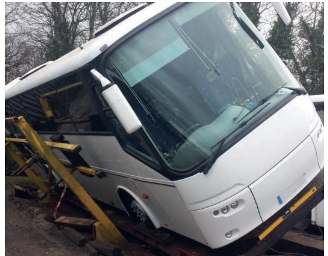
▲ Figure 1.5.33b A coach being tilted to test its stability
