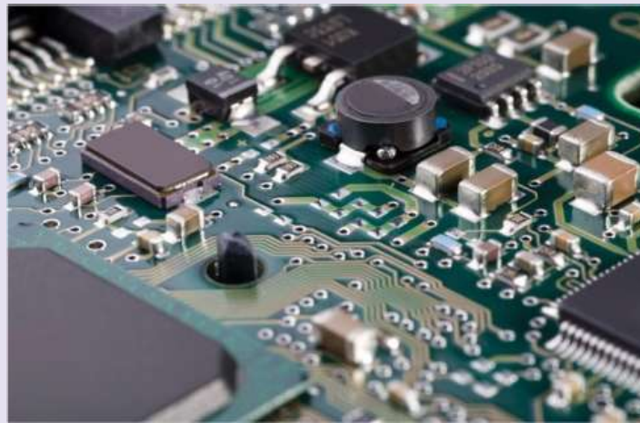
Figure 9.1: A complex electronic circuit - this is the circuit board that controls a computer's hard drive.
