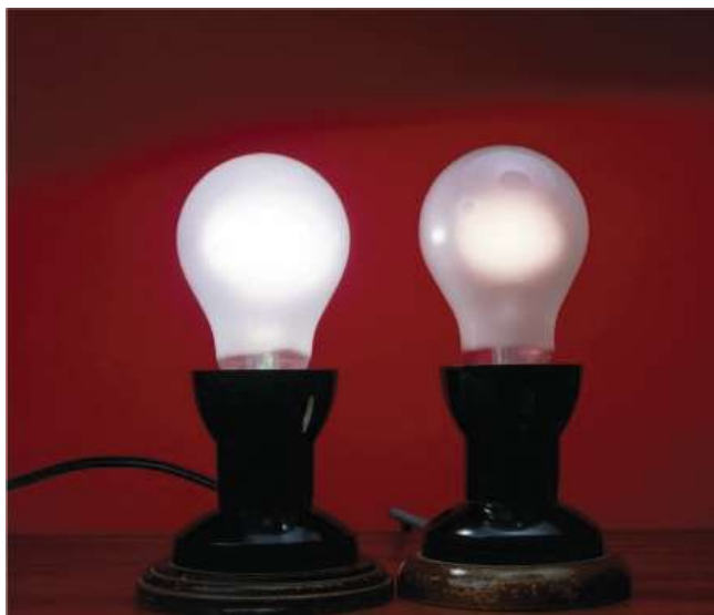
Figure 8.13: Both of these lamps work from the 230 V mains supply, but one has a higher resistance than the other. For Question 13.
