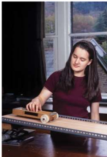
Figure 4.9: This student is investigating the acceleration of a trolley down a sloping ramp.
