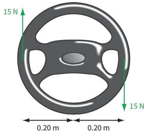
Figure 4.25: Two forces act on this steering wheel to make it turn.
