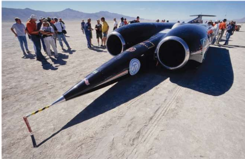
Figure 3.7: The Thrust SSC rocket car broke the world land-speed record in 1997. It achieved a top speed of 763 mph (just over 340 \text{ m s}^{-1} ) over a distance of 1 mile (1.6 km).
