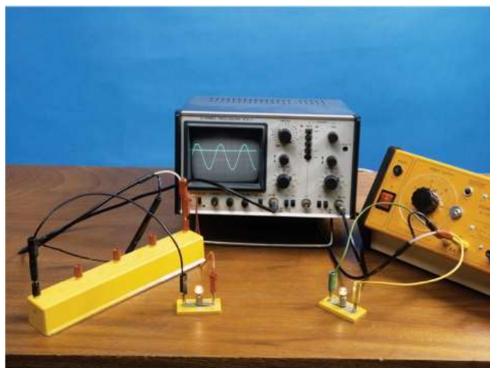
Figure 27.8: Comparing direct and alternating currents that supply the same power. The lamps are equally bright.
