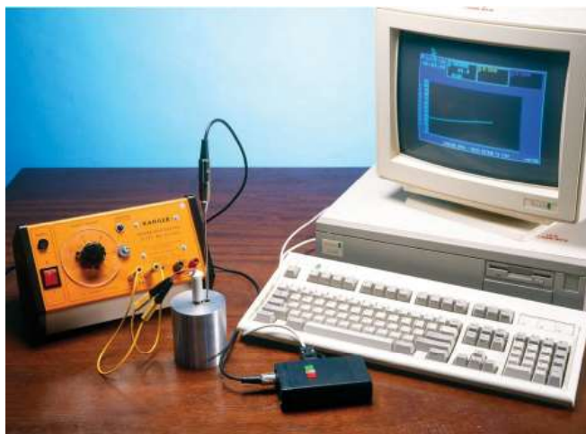
Figure 19.14: A practical arrangement for determining the specific heat capacity of a metal.
