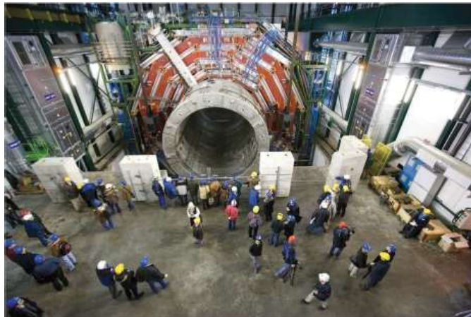
Figure 15.16: Particle accelerators have become bigger and bigger, accelerating particles to higher and higher energies as scientists have sought to look further and further into the fundamental nature of matter. This is one of the particle detectors of the Large Hadron Collider (LHC), as it was about to be installed. The entire collider is 27 km in circumference.
