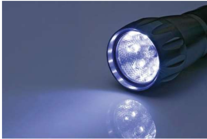
Figure 10.8: This torch has seven white LEDs, giving a brighter, whiter light than a traditional filament lamp.
