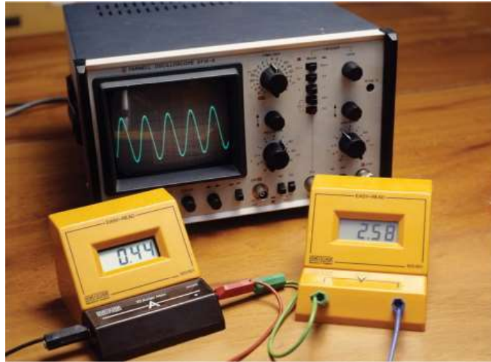
Figure 9.23: Electrical measuring instruments: an ammeter, a voltmeter and an oscilloscope. The oscilloscope can display rapidly changing voltages.
