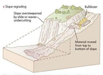
Figure 9.33 Engineering techniques for slope stabilisation
