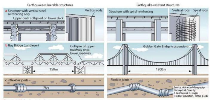
Figure 9.13 Aseismic design
