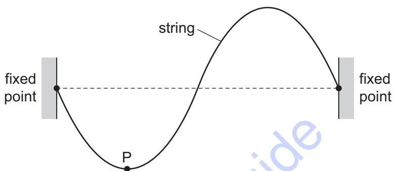
The frequency of the wave is 250 Hz. Point P on the string has a vertical displacement of  $-1.0 \text{ mm}$ .
