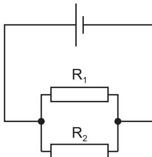
The diameter of  $R_2$  is half the diameter of  $R_1$ .
