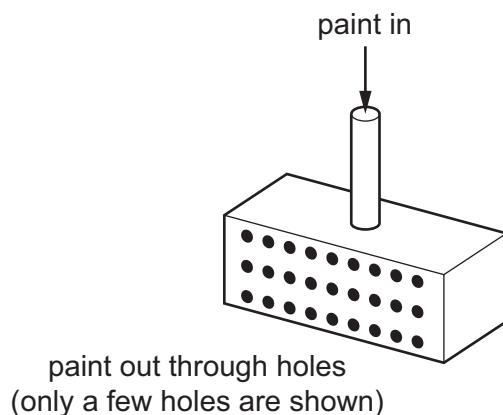
The paint is ejected at a speed of  $2.5 \text{ m s}^{-1}$  through 400 holes, each of area  $0.4 \text{ mm}^2$ . The density of the paint is  $900 \text{ kg m}^{-3}$ .
