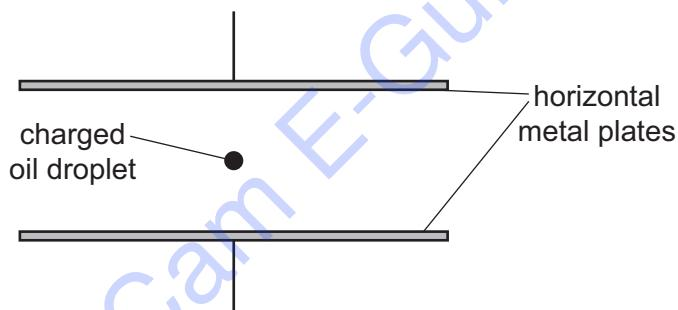
As some of the oil evaporates, the droplet loses mass and starts to accelerate. Its charge remains constant.
