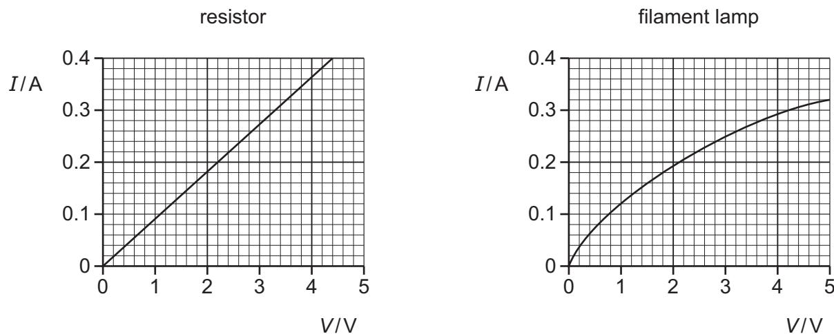
The potential difference (p.d.) across the resistor is 3.3 V.
