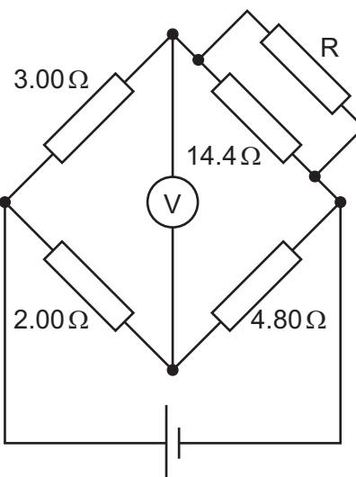
The reading on the voltmeter is zero.
