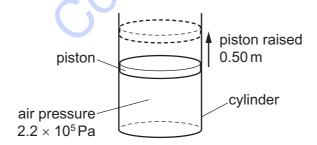
The expansion of the air causes the piston to rise through a vertical distance of  $0.50\,\mathrm{m}$ , doing 11 kJ of work. Frictional forces are negligible.
