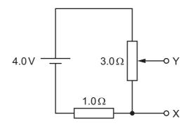
Which range of potential differences can be obtained between the terminals X and Y?
