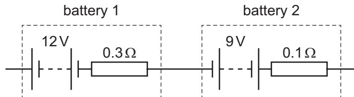
Battery 1 has electromotive force (e.m.f.) 12V and internal resistance  $0.3\Omega$ .
